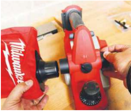
▲ The supplied dust bag can fit to either side of the planer
